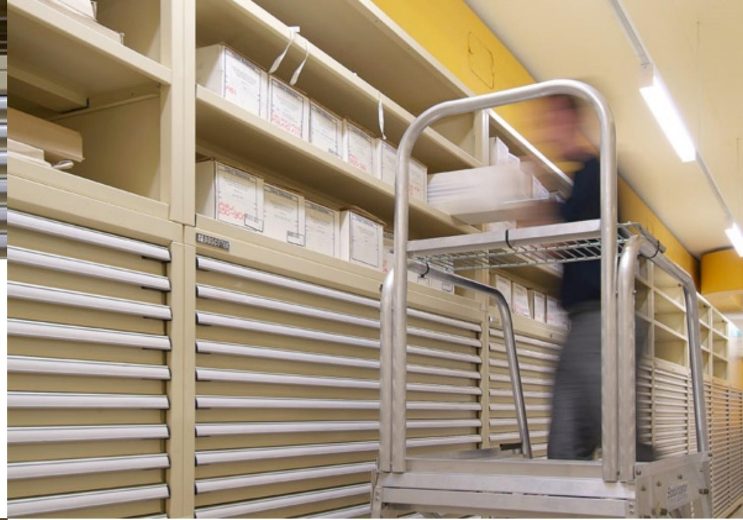
fitting A0 size maps and weighed over 900kg. This custom configuration allowed efficient and organised archive storage that was quick to retrieve with total map visibility for staff working in the archives. The specification required the additional feature of a specially designed rear hood and hinged front flap to protect the contents in each drawer.
